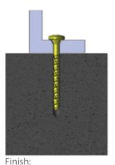
The anchor must be snug after installation. (Note: To retain values, anchors may not be loosened or removed and reused after installation.)
