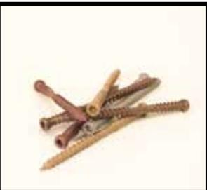
**Kameleon™ Composite Deck Screws:** Heads blend in with decking with no mushrooming effect. Use in plastic or composite decking. They are available in; Grey, Tan, Brown and Redwood. The Kameleon screws are self tapping featuring fiber trapping rings, a countersinking head with cutting teeth, CEE Thread™, W-Cut™ threads for reduced torque and our Climatek™ AC257 code approved coating. They are ESR code approved under ICC Report ESR-3201.
